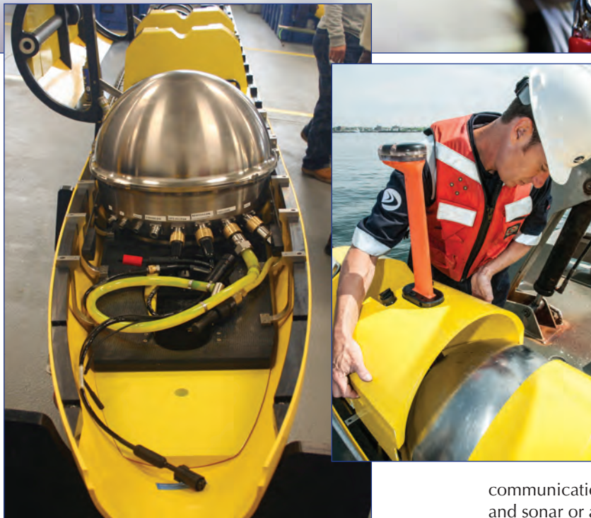
(Top) Minute BIRNS Millennium 3G connector (0.33-inch) insert during rigorous continuity and insulation resistance testing procedures. (Bottom Left) BIRNS Millennium connectors served as the primary connector type for the AUV's main electronics housing (MEH), the air-tight pressure vessel where system-critical electronics reside. (Bottom Right) Bluefin marine operations engineer removing foam to gain access to the MEH.
